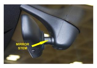
**STEP 3** - While sitting in the passenger seat, place the mount over the mirror stem. Tighten the CLAMP SCREW until the mount starts to clamp onto the mirror stem. Position the mount as far forward as it will go and paralell to the bottom of the mirror before fully tightening.
